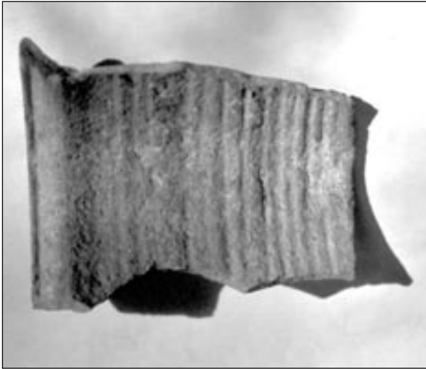
Figure 10. Typical rippled wall pattern within the interior of Nabataean piping.
